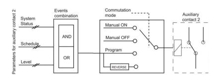
The auxiliary contacts react to different types of signals,
