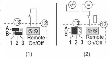
Contact by a voltage (max. 60V eff. / 30mA): the jumpers are set as in (2) A1-B1 and A2-B2.
