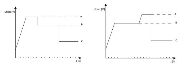
A= equalization voltage, B= absorption voltage, C= floating voltage
